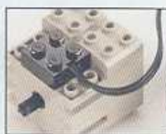
With the wire attached this way, the motor turns one direction.
